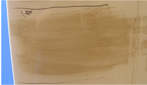
Figure 14: Modified Lower Surface Oil-Flow Image
