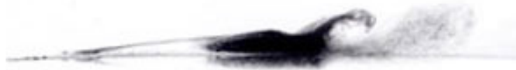
Figure 1: Smoke Image of Transition from Laminar to Turbulent Flow (Greg Cole and Prof. Mueller, Notre Dame)
